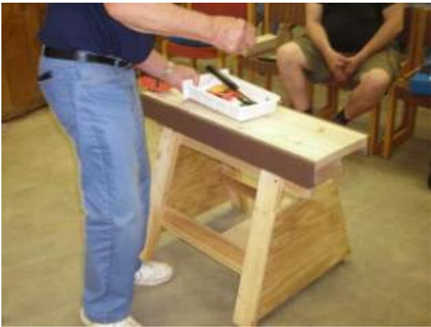
Portable workbench mounts on top of the sawbuck.
