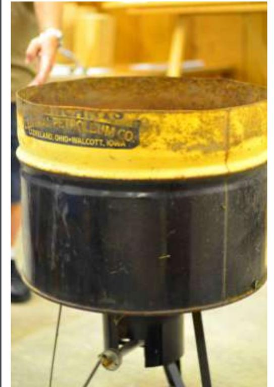
For boiling wood bowls and other pieces, Brian uses a cut off 55 gallon barrel sitting on a gas burner you can get at a camping store for about \$20. It hooks up to propane.
