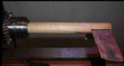
Mandrel made from dowel: 3/8" and 5/8" dia.
