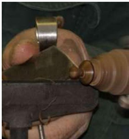
The globe was hollowed out to a thickness of 1/16" to 1/8". Rick used a special hollowing tool with an outrigger that prevented twisting of the tool in the turner's hand.
