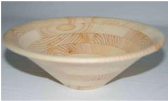
Dick Fornasierre made a stacked ring bowl by tilting his bandsaw at 45 degrees and making semi-circular cuts.
