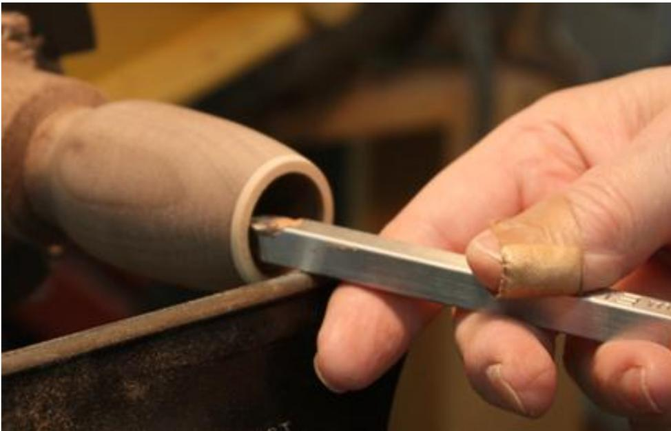
I've started hollowing the goblet using the finisher, working from the top down towards the base. I take small cuts being careful not to get catches or excess tear-out inside the goblet. I want the walls to be around 1/16" or less. I use a
