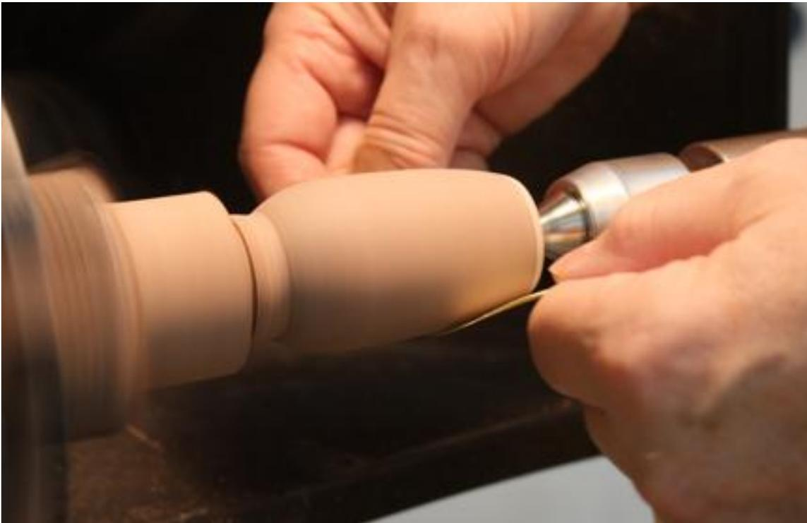
I've sanded the outside to about 400 grit. I still have quite a bit of wood supporting the bottom of the goblet.
