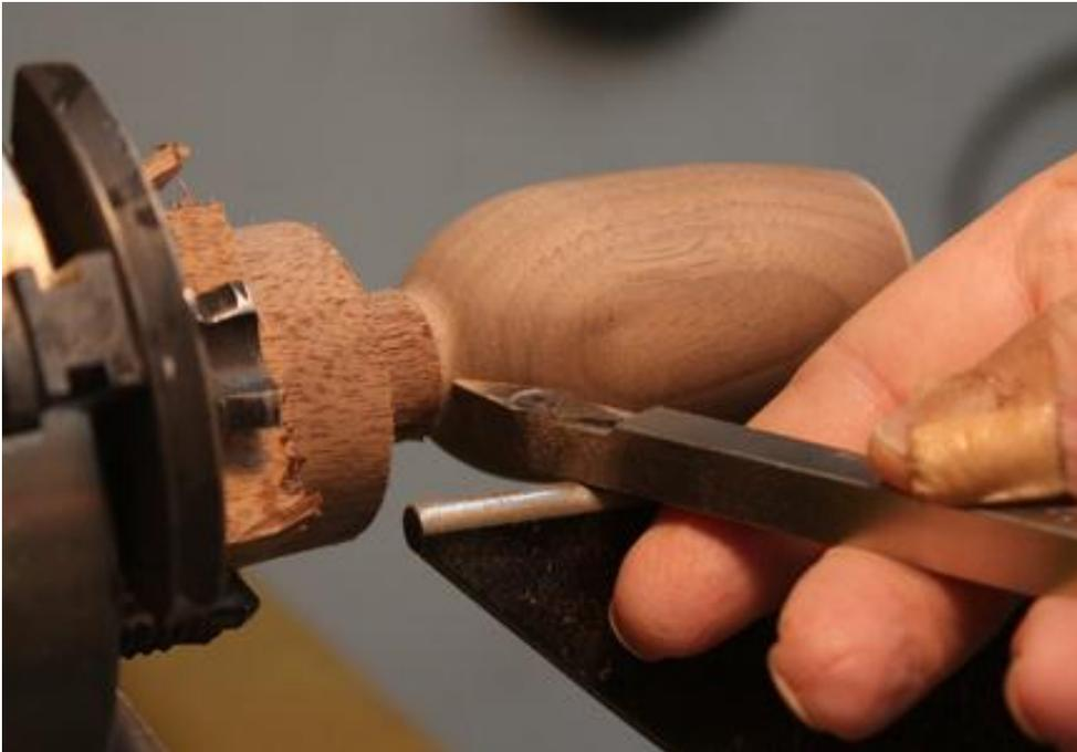
Here I'm taking the bottom to finished roundness a little at a time, keeping as much wood as possible at the headstock end.
