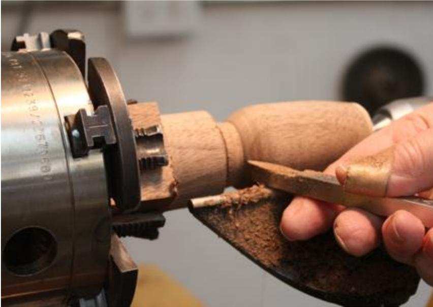
I've shaped the top of the goblet and am partially turning the bottom curve. Note that I didn't remove much wood from the headstock end of the blank so I have a good support and enough mass when I work on the inside of the goblet.
