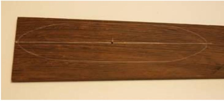
The outline of the top has been traced on the blank, here a 1/8" piece of wenge. I've drawn a line through the center, using marks I made where the center spline is located. I divided the line in half and marked where the center of the hole will be.
