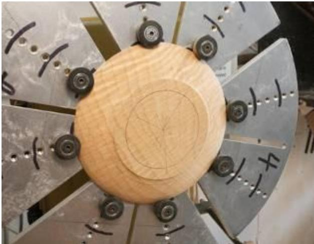
I've now reversed the blank and mounted it to a set of Coles jaws. This will allow me to finish turn the outer face without having to use an elaborate vacuum chucking system and I can leave the tailstock out of the way. You could also make a large jam chuck, but the Coles jaws are much simpler to set up.
