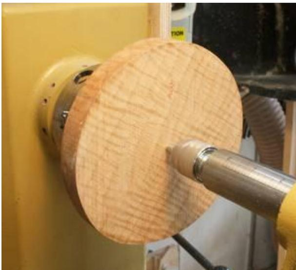
I've drawn up the tailstock live center to secure the blank. Since the blank is held in place with just the double sided tape, I don't want to take any chances that it will fly off the lathe. Now I'll turn the blank round and start working on the general outside shape.
