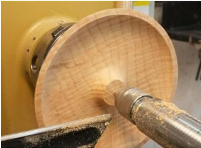
Most of the inside of the vessel has been turned away. Note also that I've kept the tailstock engaged for safety reasons. I don't want to take a chance of the turning coming loose from pressure placed on the outer edges of the bowl where there's no backing support.
