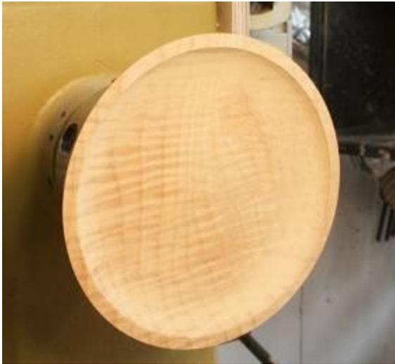
The inside of the vessel has been turned with a wall thickness of around 3/16". The thickness isn't critical. It should be thin enough to resist cracking and give the finished piece a light feel but you don't have to try to impress anyone with how thin you can make the walls. Since it'll be covered completely when assembled, there's no need to do any sanding. Note that the rim is fairly wide to provide an adequate gluing surface.
