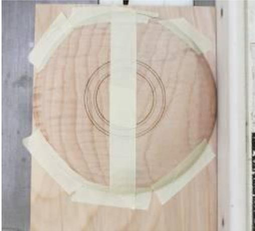
The vessel has been secured to the carrier with masking tape and is ready to go. This is a one-time operation so the masking tape will be more than sufficient to secure the vessel. Note that I've taped the area where the blade will cut. This will help control any chipout, especially at the back edge. Grain orientation is important here, and generally it's better to have the grain running the same direction as the saw cut.
