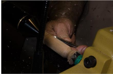
*Mark is using a gouge to bring the lure into shape*
