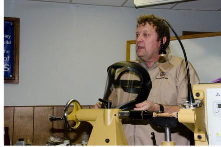
*Note the full face shield, including neck coverage with a high impact resistance plastic*
