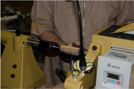
*Roughing the blank to a cylinder - note this is spindle work so a roughing gouge is acceptable*
