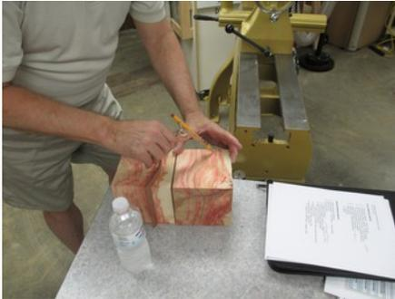
*Rich is scribing an arch on the top block, the bottom block has already been though, bubinga inserted and been glued up*
