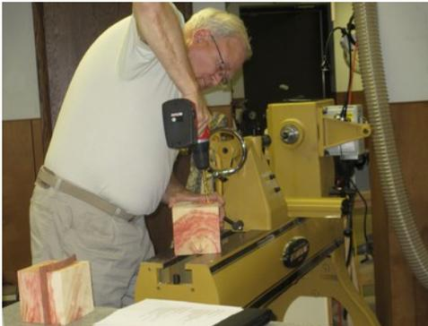
*Here a hole is being drilled through the block for the dowel*
