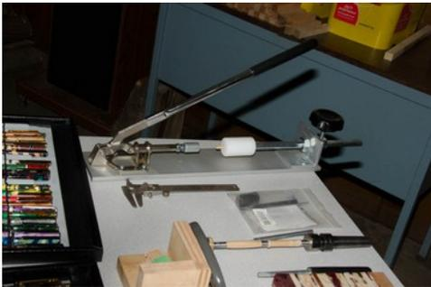
*From top to bottom: Assembly press, caliper, pen kit, pen mandrel (with mounted blanks), and a drilling jig.*
