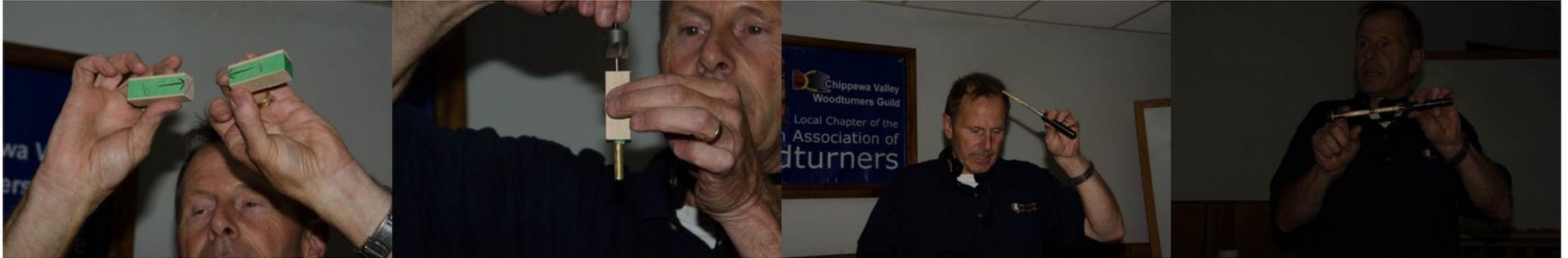
Note the painters tape with arrows pointing out orientation. Bruce maintains this orientation on the mandrel.
