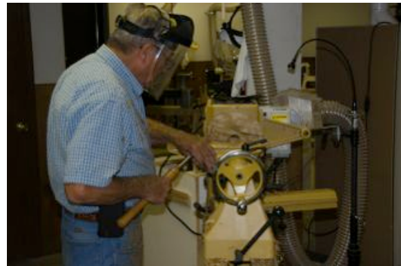
Figure 2 - Joe is surfacing the blank.
