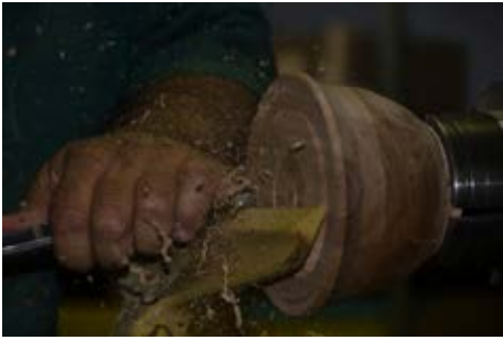
BOWL MOUNTED IN JAWS FOR ROUGHING
