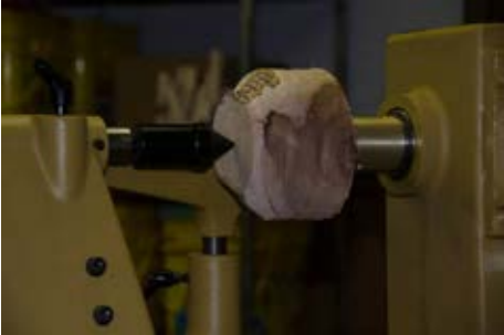
WOOD MOUNTED BETWEEN CENTERS
