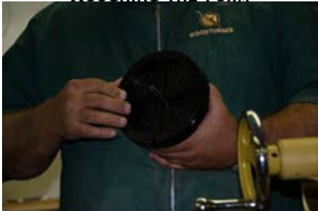
EXAMPLE OF A SCREW CENTER
