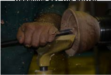
INCH BY INCH TO FINAL THICKNESS
