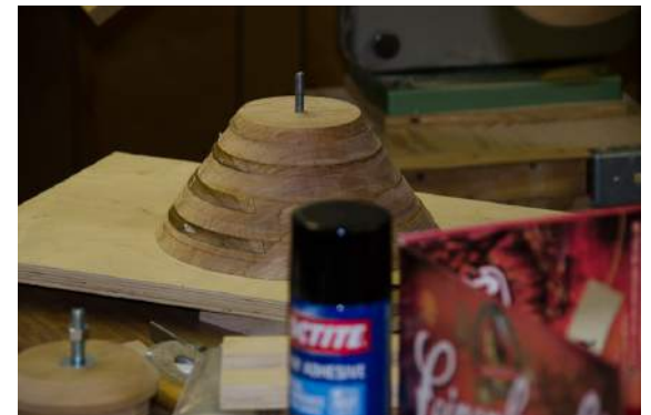
Gluing jig, pressure applied by nut and washer.
