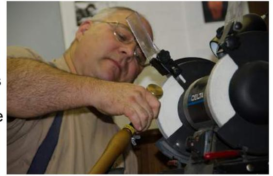
material from the bevel the side grinds should be completed first, then in a single pass, sharpen the bevel. To maximize the life of the tool (or minimize the amount of metal being ground away) it's important to always have the same amount of tool sticking out from the vari-grind, such as 2". Read your tools documentation to find their recommendation. A good practice is to drill a 5/8" hole in a piece of wood to the proper depth and use that to set the tool in the vari-grind.
