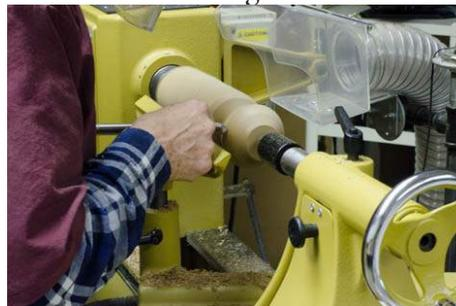
**SHEAR CUTTING WITH GOUGE**
