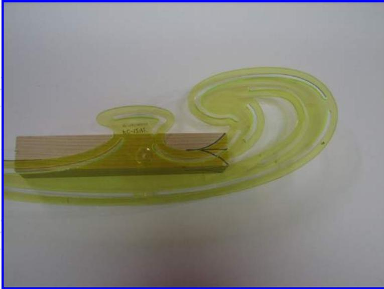
Use a scroll saw, coping saw or similar tool to cut along the “V” shaped curves you have just drawn.
