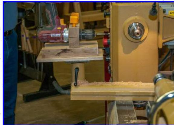
**One of Joe's homemade jigs to drill measured hole distances using the index function on the lathe.**
