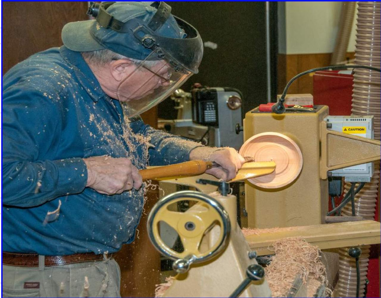
**Joe Nycz demonstrates technique for turning a small bowl and chucking types**
