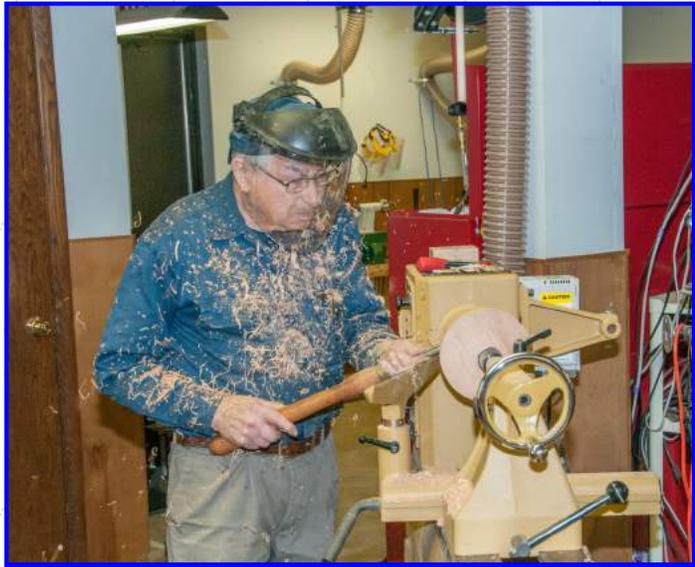
He then used a carbide scraper to rough the wood into a round shape. A bowl gouge could also be used for this, but a spindle roughing gouge (and all roughing gouges are spindle roughing gouges) can not. A spindle roughing gouge has a tang which represents a weak point. In the event of a catch it is likely that the tool will break at this point. Avoid injury, only use proper tools for work where the grain is perpendicular to the bed.
