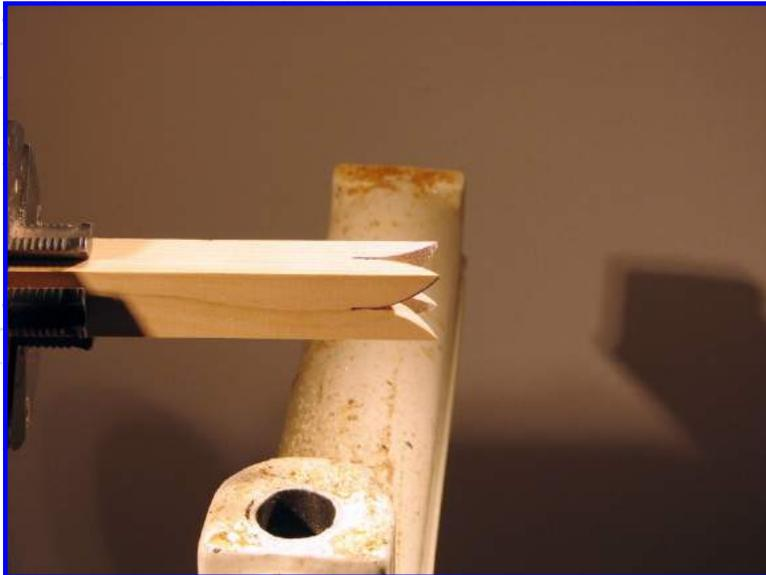
Using a sharp spindle gouge delicately turn the flower shape starting at the very tip of the flower. The tip has only a small amount of wood that needs to be removed. Proceed with care! Further down the flower there is more wood to be removed. With the wood spinning it is easy to see the cut out shape of the “V” that will help you gauge when the profile is “OK”.
