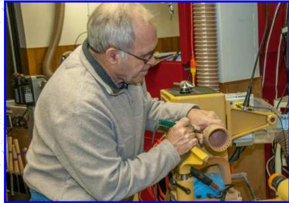
Wendel draws reference marks on his piece. First he uses the indexer to draw lines parallel to the bed. He then draws vertical lines around the circumference with the lathe on slow. This helps to keep the pierced details symmetrical.
