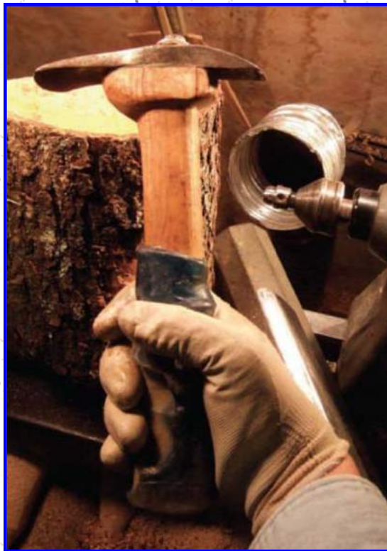
Figure 1. Hand adze that the author made for stripping bark from a piece to be turned.
