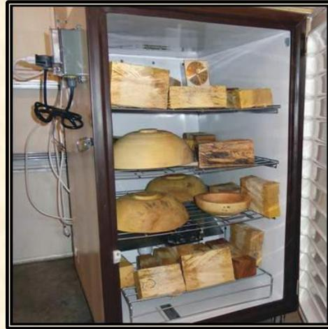
To speed up the drying process and improve the odds of successfully preserving wood blanks, I built a drying kiln. A kiln provides a stable environment by maintaining a consistent temperature and humidity. For research, I spoke to woodturners in my local club and also found articles on the Internet. I discovered that there are no hard-and-fast rules for building a kiln, so I took several ideas and combined them into something that would work for me.
