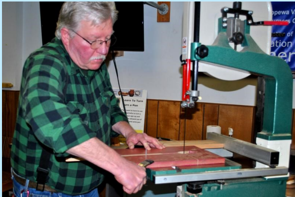
Left: Setting up the shop made circle cutter.
