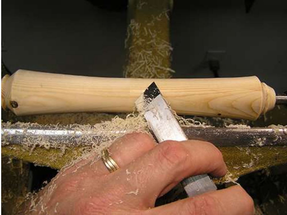
Cutting a long, shallow cove with the skew. Notice the smooth surface left on this pine.
