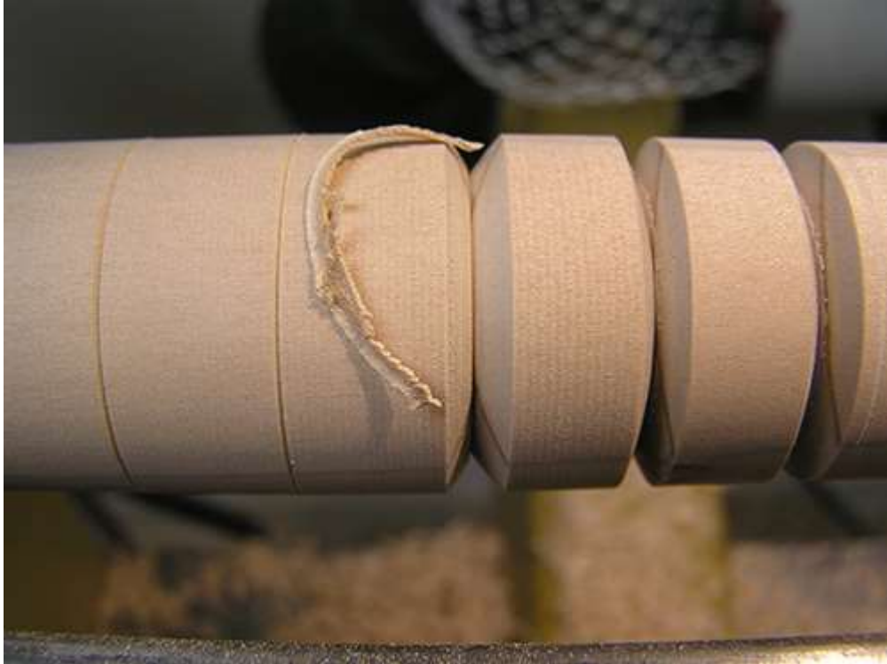
The circular chip that results from a V-groove cut.
