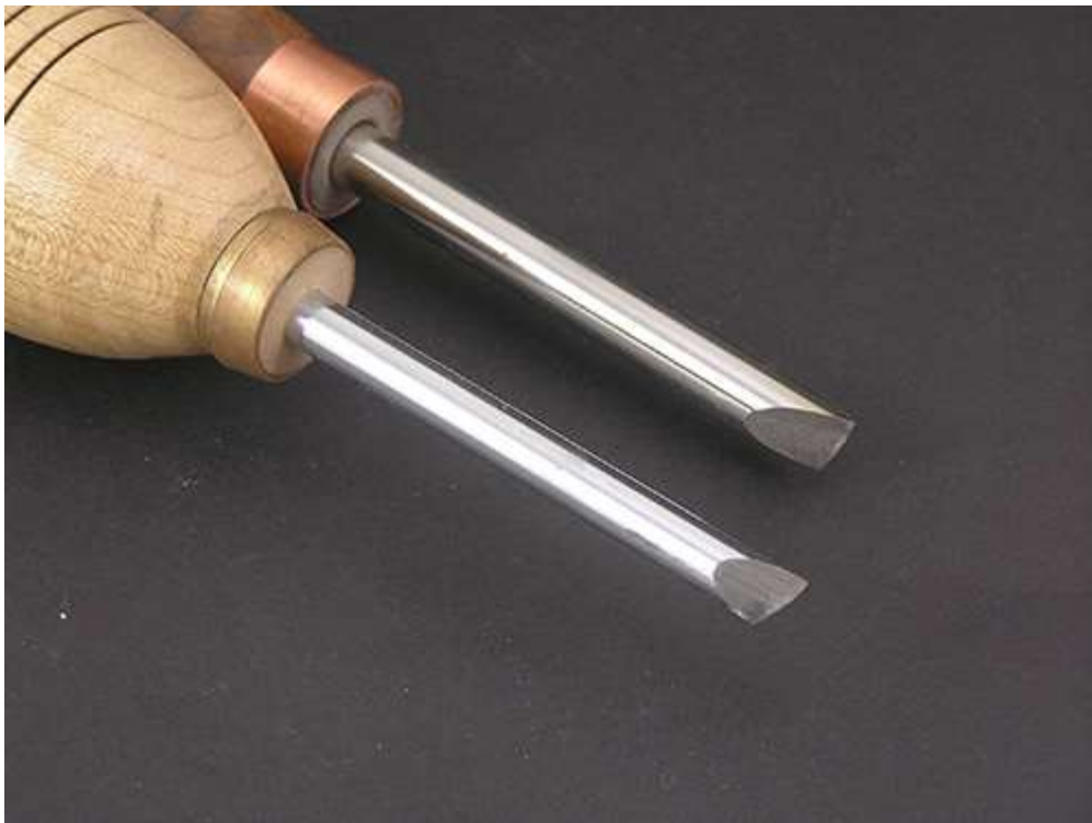
Rectangular skew with both top and bottom edges rounded.
