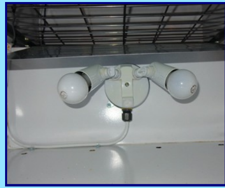
The lightbulbs are mounted on the back of the kiln near the bottom, a sheet of metal covers the bulbs and the holes are drilled through the bottom of the freezer.
