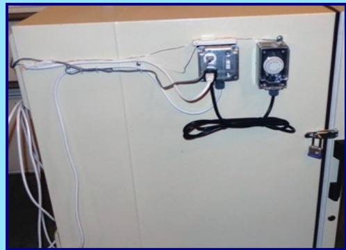
Mounted on the left-hand side of the kiln are the controls, power switch, and outlet, as well as the greenhouse controller. Note the padlock for safety.
