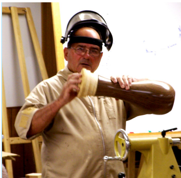
Barry dyes the turned demonstration piece with a liquid Rite dye.
