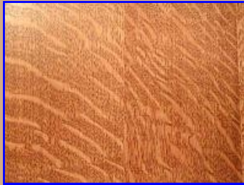
Quarter sawn wood showing pattern of rays (whitish streaks)
