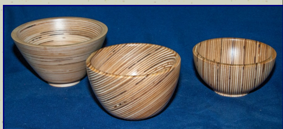
Mark Palma with 3 Baltic Birch plywood bowls turned in different grain orientations. Also a small plate turned from “architectural foam” (aka PVC).
