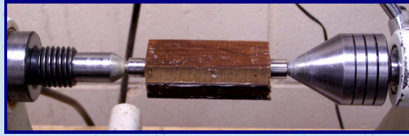
Mounted blank between centers on stepped bushings
