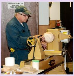
Placing bowl on the vacuum chamber
