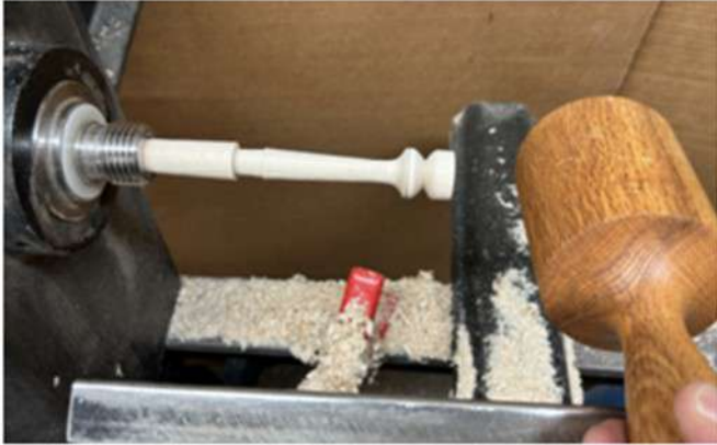
Fig 17a Firmly pound the peg blank into the headstock. Fig 17b|Bring up the tailstock for additional support initially.
