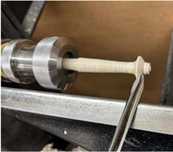
Fig 15a. Turning the bead on the head with a spindle gouge after backing off the tailstock live center.
