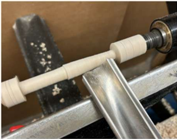
Fig 8a. Remove bulk of peg taper with roughing gouge.
