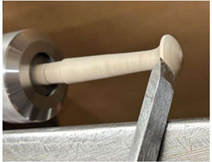
Fig 15b. Turning the bead on head with a skew.
