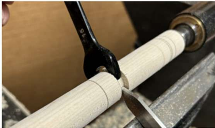
Fig 4a. Reducing the peg shoulder to 19/32 " (15mm)
