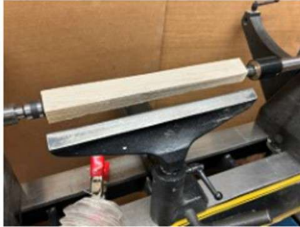
Fig. 1 Mounted hardwood blank.
