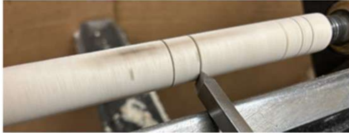
Fig 3. Marking penciled lines with skew V cuts.
