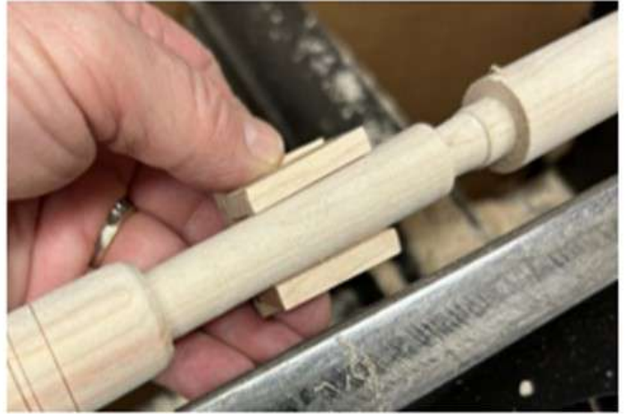
Fig. 7. MT2 Taper to jam in spindle.
