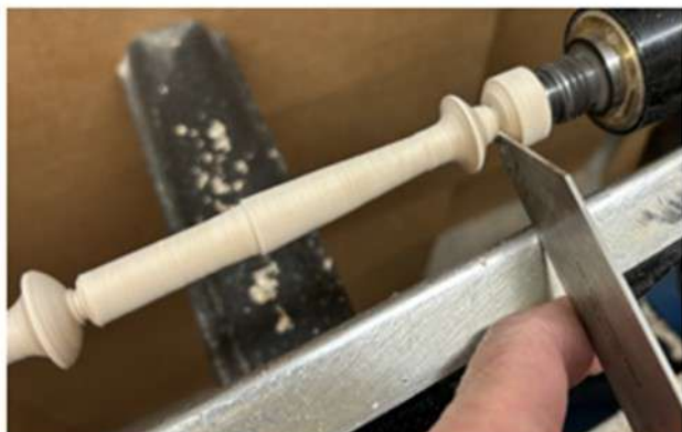
Fig 11a. Partial part off before sawing.
