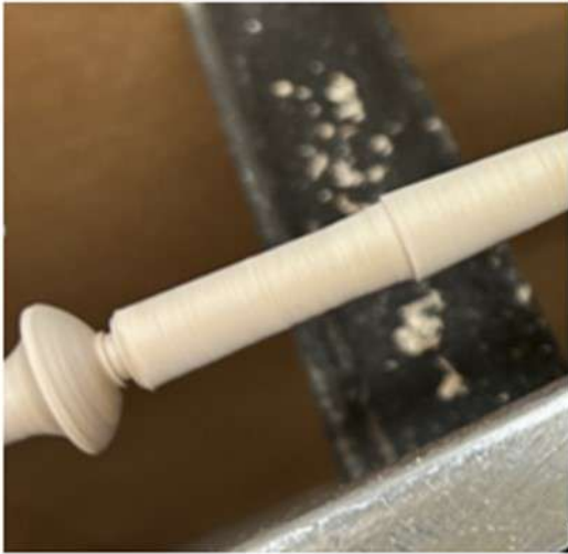
Fig 6. Longer 1/2" tenon for in collet chuck.
