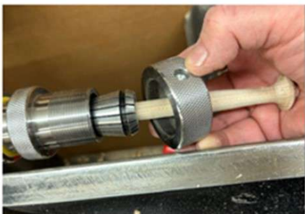
Fig 12a. Mounting the tenon into the collet chuck.
