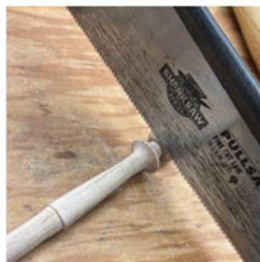
Fig 11b. Separating with a saw.
