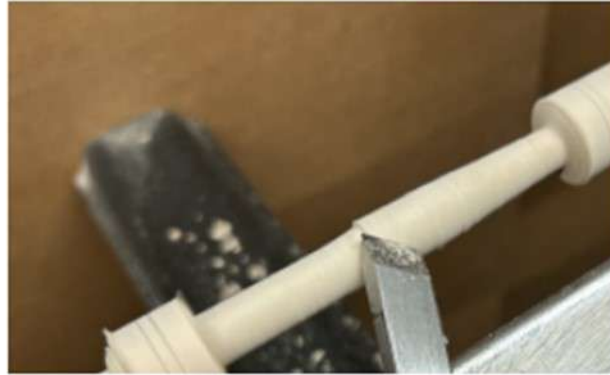
Fig 13. Putting a nice finish on the Peg's taper with a skew. You can also use a spindle gouge.
