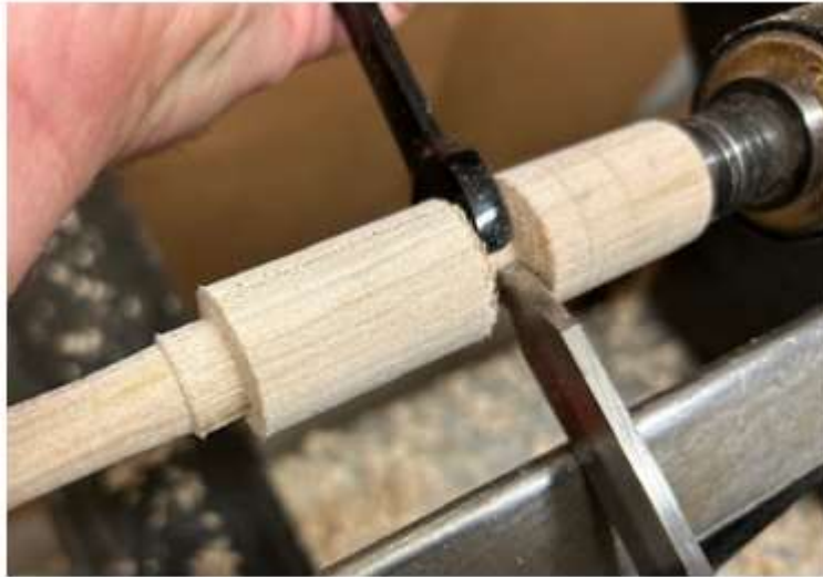
Fig. 10 Reduce the peg neck to 7/16'' (shooting for 3/8'' final). This image was done before reducing the bulk of the peg's taper.
