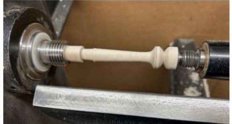
Fig 17a Firmly pound the peg blank into the headstock. Fig 17b Bring up the tailstock for additional support initially.
