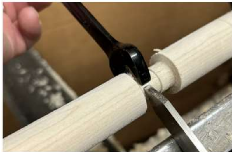
Fig 5. Reduce the peg tenon to 1/2 " with a taper ( 31/64 " to 33/64 " at the shoulder using a 1/2 " wrench at the tenon's midpoint.
