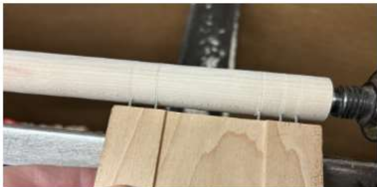
Fig 2. Marking the spindle with key points, using a card or a measuring jig with nails.
