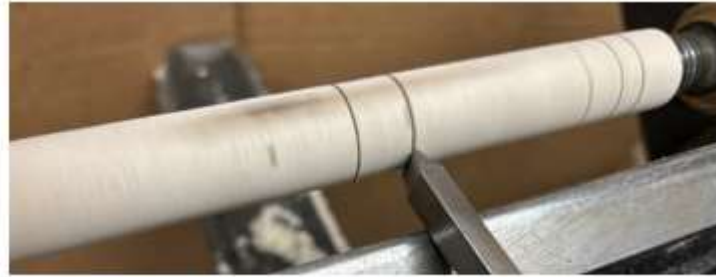
Fig 3. Marking penciled lines with skew V cuts.
