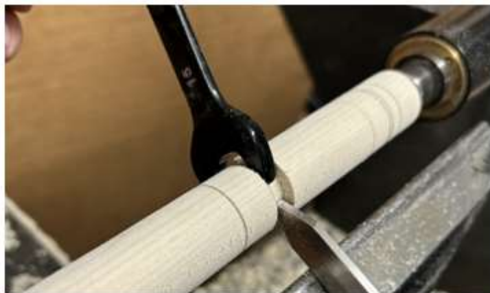
Fig 4. Set depth of the shoulder of the peg's tenon to 19/32 " (15mm)
