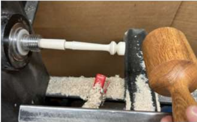
Fig 17a Firmly pound the peg blank into the headstock. Fig 17b Bring up the tailstock for additional support initially.
