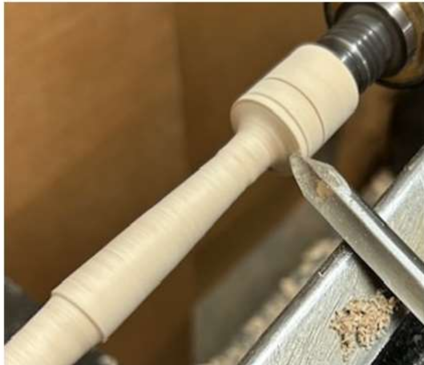
Fig 14. Turn \frac{1}{2} cove with a spindle gouge, smoothly into the peg's taper. If you're brave try doing it with the skew.
