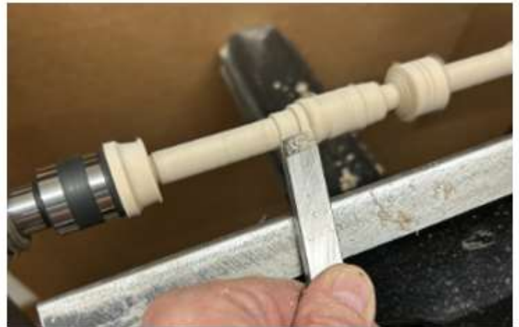
Fig 8b. Removing bulk of peg taper with skew peeling cuts.
