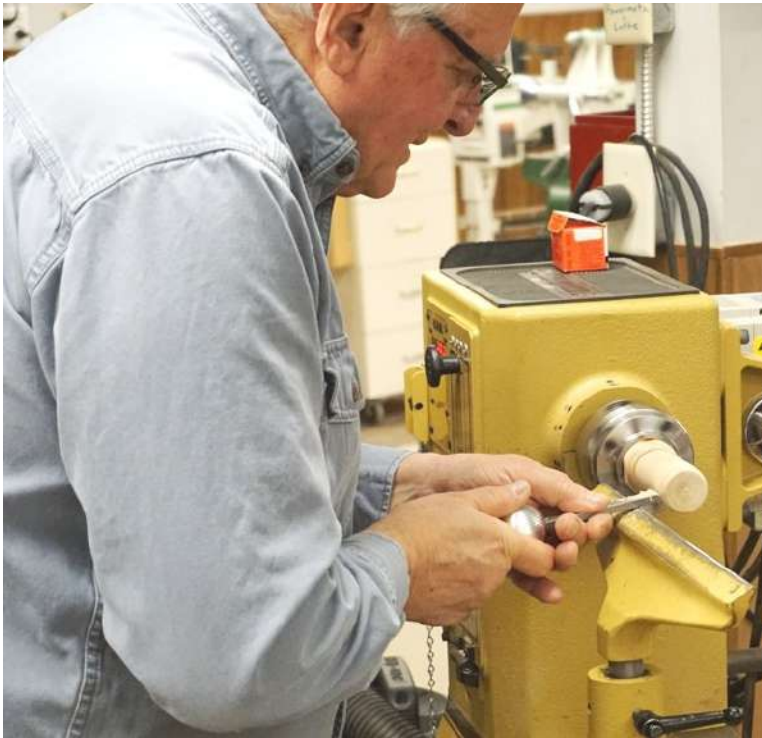
Tom using the external thread chaser. He went over the threaded area several times pressing in a little further each time to get a final thread cut.
