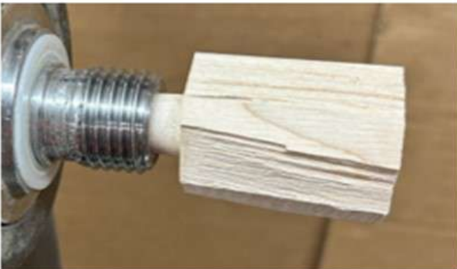
Fig. 4 A blank turned between centers to have an MT2 taper and tapped into the headstock.
