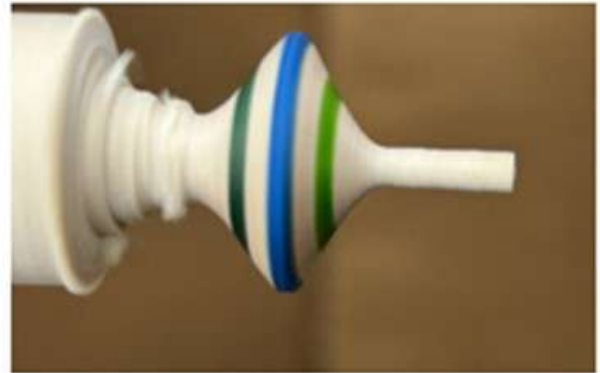
Fig. 7 A top turned with the handle on the free end. Only the turning point remains to be finished.
