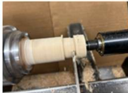
Removing the material around the handle with a parting tool.
