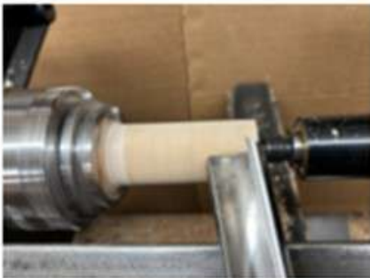
Turning a cylinder.
