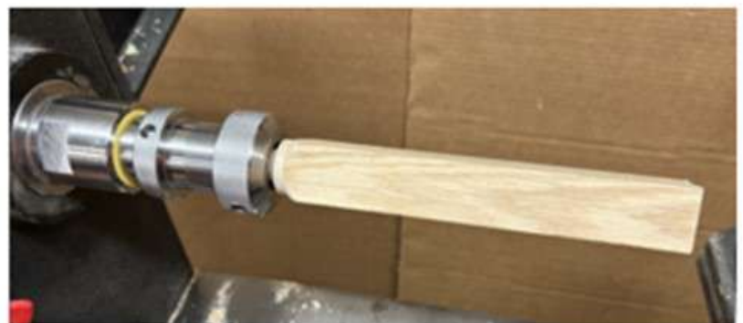
Fig. 5 A blank turned between centers with a tenon that can be supported in a collet chuck.
