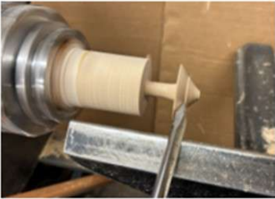
Fig. 8 Forming the point with the tailstock removed.
