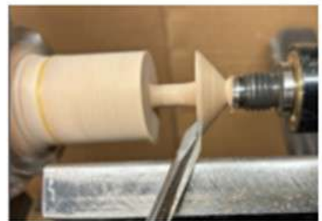
Starting to form the top's bottom.
