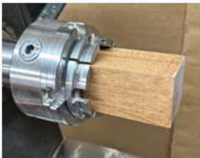
Fig. 1 A square blank of a size that can be mounted in a chuck.
