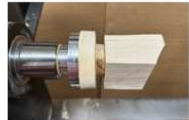
Fig.3 Glued to small board, mounted on a faceplate.
