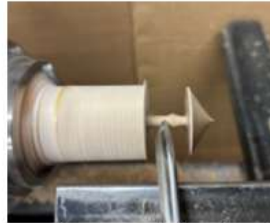
Fig. 9 Cleaning up the handle and top surface.
