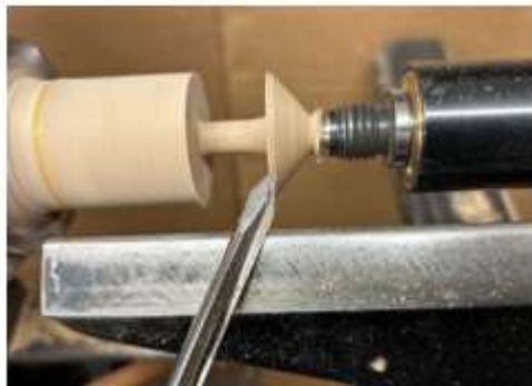
Fig. 6 Supported by handle on right side and forming the turning point on the left.
