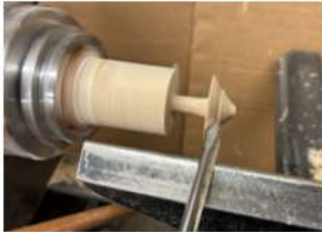
Fig. 8 Forming the point with the tailstock removed.
