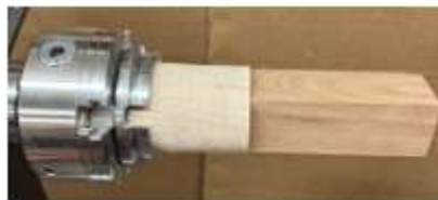
Fig. 1b & 2 Glued to a round blank, mounted in a chuck.
