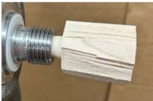
Fig. 4 A blank turned between centers to have an MT2 taper and tapped into the headstock.
