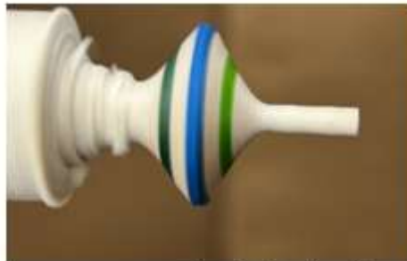
Fig. 7 A top turned with the handle on the free end. Only the turning point remains to be finished.
