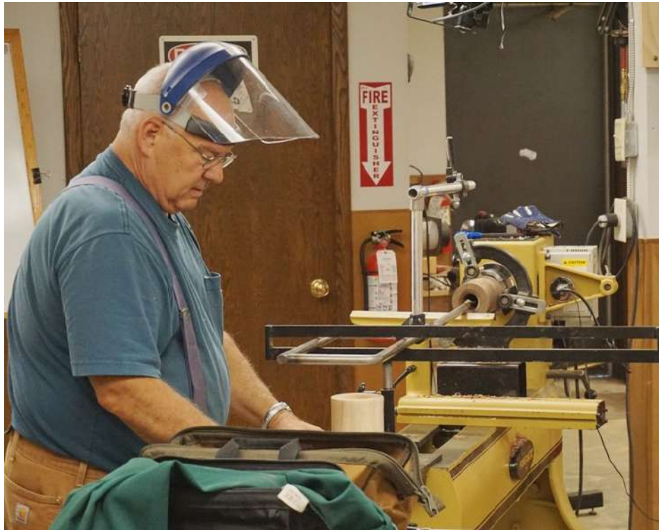
Bob setting up the Jamieson System of Hollowing
