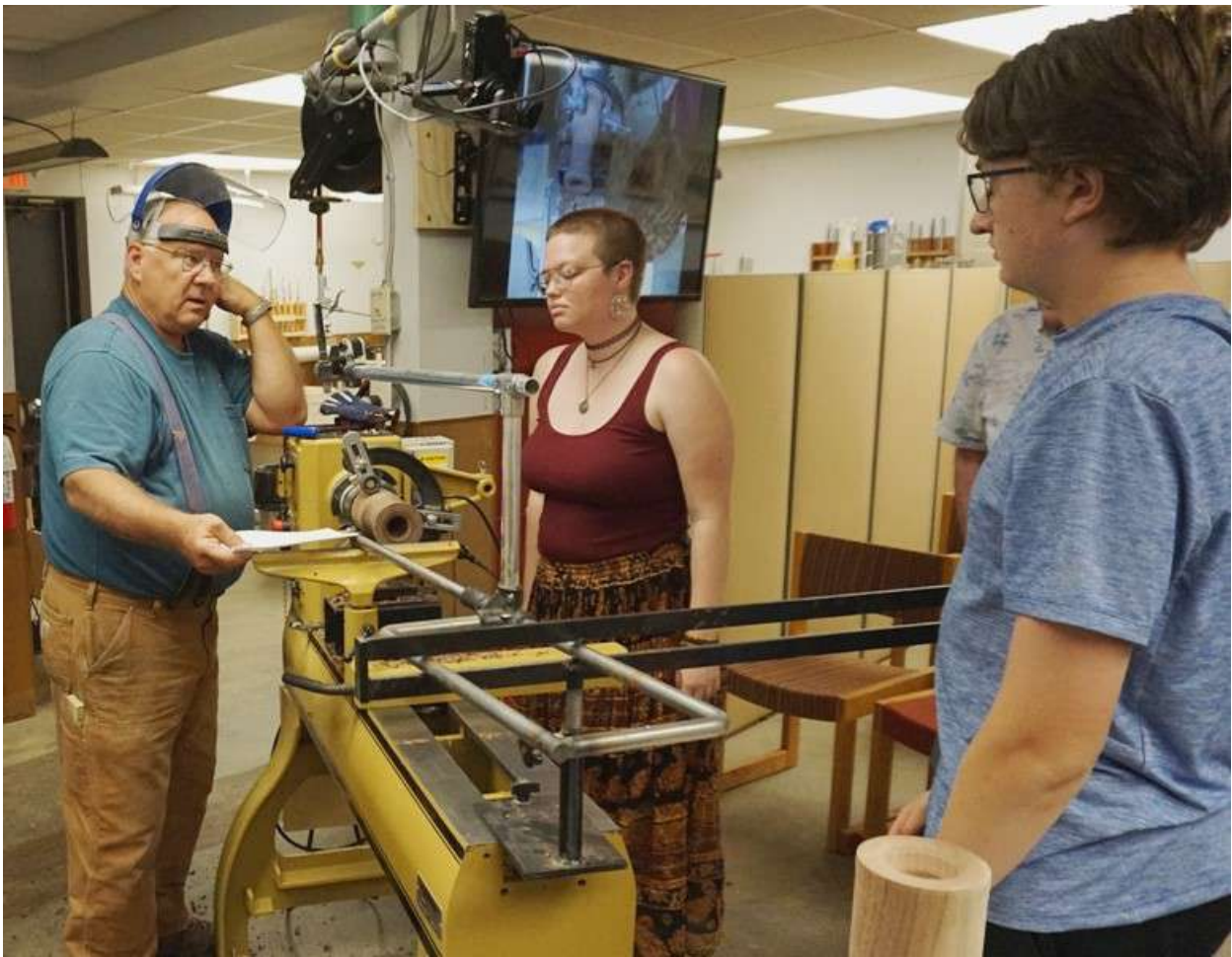
Bob demonstrates to members how a depth laser works . This involved setting the laser to a certain depth and Bob moved the hollowed blank back and forth to show how the laser dot elongates after reaching the desired depth.
