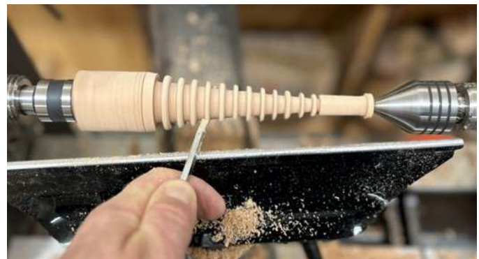
Figure 6, Turn the edge of each ring to a bead.
