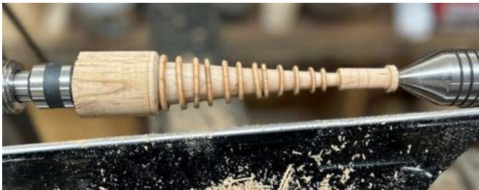
Figure 11, Once rings are free, smooth the cone behind the rings with a skew. Check spacing and adjust the cone as needed.
