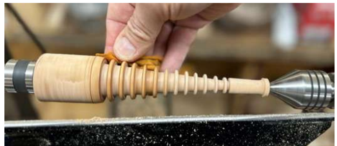
Figure 8, Apply a finish to the rings you just sanded.
