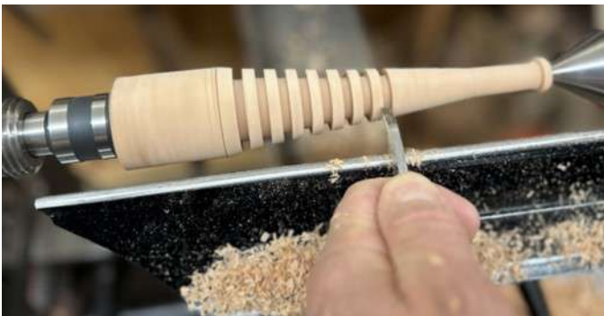
Figure 4, Using parting tool, form the rings.
