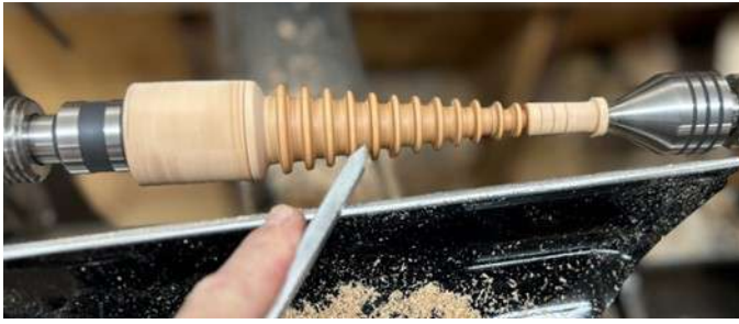
Figure 9, Begin parting off each ring. Here using a skew and 3 light cuts from each side. You have to start at the smallest ring.
