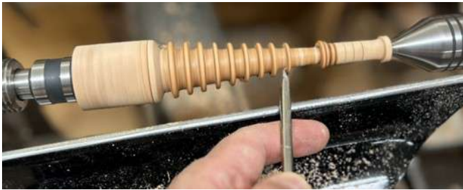
Figure 10, Here I'm parting off with a tiny hook tool I developed to scrape behind the ring for an easy parting.
