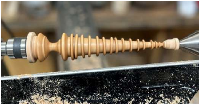
Figure 12, Next, shape the base and the small top of the tree. Apply finish before carefully parting off both ends
