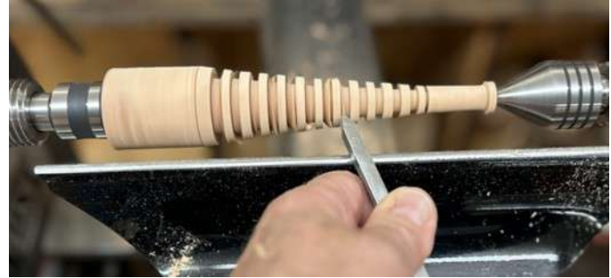
Figure 5, Use the skew to clean the end grain on both sides of each ring. This also makes the ring thinner.
