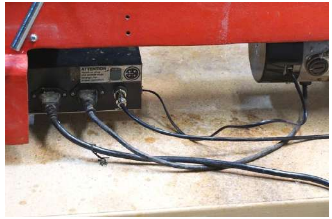
Right Above: The loose wires from the switch box. The wire on the left is the power cord. The next wire goes to the motor. The next wire is the power to the small circuit board for the light and the speed LED. The next smaller wire with telephone type connectors have something to do with the variable speed.
