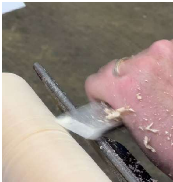
Dan demonstrating a Toe Dig-In catch with the Skew.
