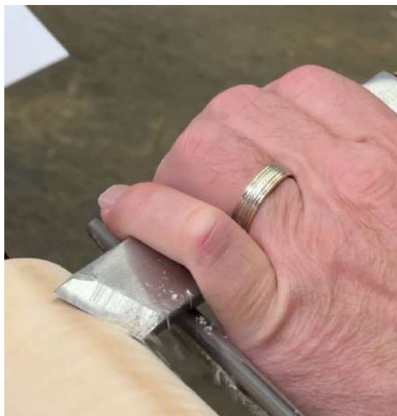
Dan demonstrated the planing position with a Skew.
