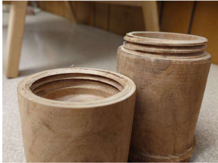
A set of Joe's coarse male and female threads. I think he said it was 5 TPI.
