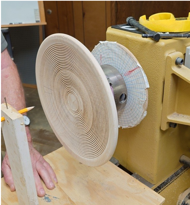
John demonstrates his segmenting indexing jig.
