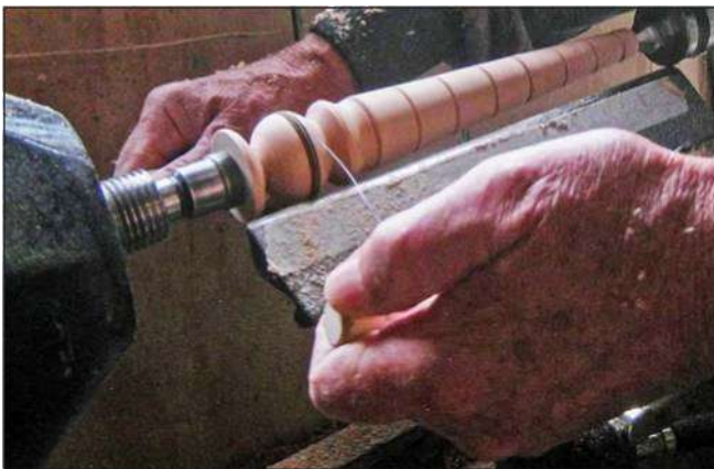
8. Use a length of wire to add decorative burn lines. The author uses a guitar's G string with handles added to each end.
