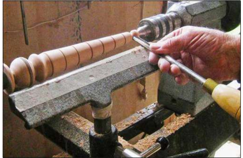
9. Round-over the bottom of the dibble, leaving about 1/4" of material attached to the waste end.
